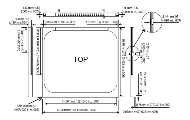
Note: The optional notched configuration was shown in the CF Specification Rev.1.0. In Specification Rev. 1.2. The notch was removed for ease of tooling.
